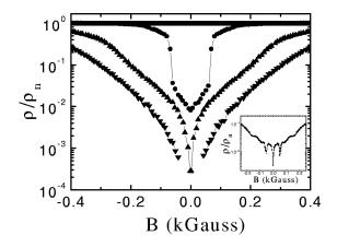
FIG. 4. Field dependence of the resistivity (normalized by the normal state value  $\rho_n$ ) at  $T=0.99T_C$  for a Nb film on a (0.4 ×0.95)  $\mu$ m<sup>2</sup> array of Ni dots (sample 2) in configuration B: squares  $J=10^5$  A/cm<sup>2</sup>, circles  $J=6.25\times10^4$  A/cm<sup>2</sup>, up triangles  $J=3.5\times10^4$  A/cm<sup>2</sup> and down triangles  $J=2.5\times10^3$  A/cm<sup>2</sup>. Inset shows the  $\rho$  vs *B* curve in configuration A for  $J=10^4$  A/cm<sup>2</sup>.
