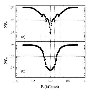
FIG. 2. Field dependence of the resistivity (normalized by the normal state value  $\rho_n$ ) at  $T=0.99T_C$  and  $J=3.1\times10^4$  A/cm<sup>2</sup>, for a Nb film on a (0.35×0.5)  $\mu$ m<sup>2</sup> array of Ni dots (sample 1): (a) geometry A, (b) geometry B.
