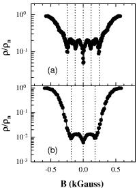
FIG. 3. Field dependence of the resistivity (normalized by the normal state value  $\rho_n$ ) at  $T=0.99T_C$  and  $J=3.7\times10^3$  A/cm<sup>2</sup>, for a Nb film on a (0.35×0.5)  $\mu$ m<sup>2</sup> array of Ni dots (sample 1): (a) geometry A, (b) geometry B.
